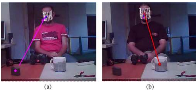
Fig. 9. Estimated gaze direction and object depth via GP regression (line) together with the center of the manually annotated object of interest (solid dot).
