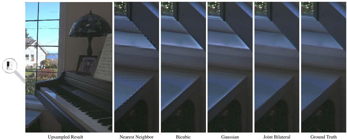
Figure 2: Tone Mapping: The low resolution exposure map solution at left is at scale relative to the final upsampled result next to it. Detail insets to the right show results from Nearest Neighbor, Gaussian Interpolation, Bicubic Interpolation, Joint Bilateral Upsampling, and ground truth based on a full resolution solution. Note that JBU does not exhibit the blocking and halo artifacts of the other upsampling methods.
