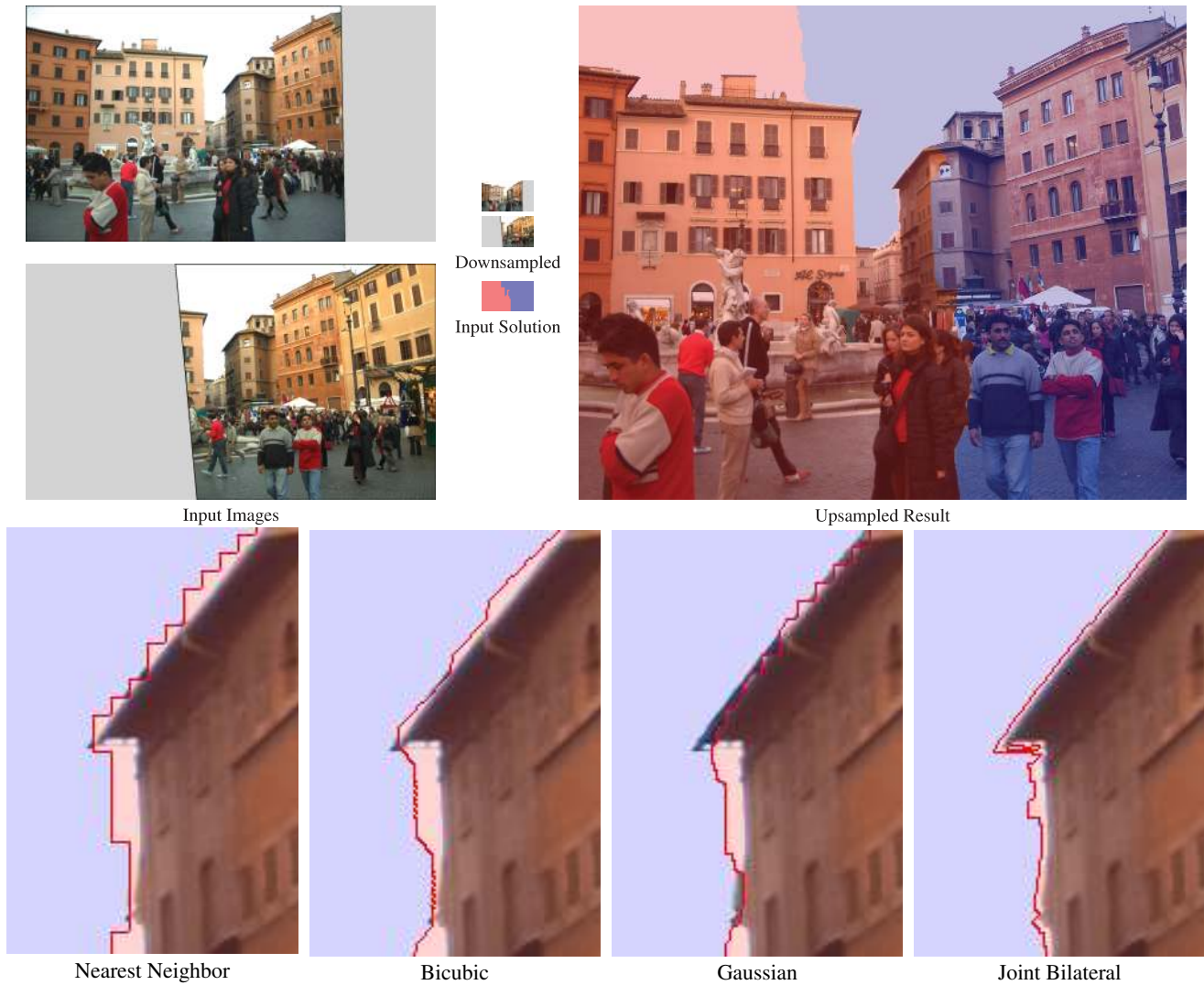
Figure 5: Graph Cut based Photomontage. Upper left: two original aligned images. Upper center: the downsampled images and the resulting labeling solution. Upper right: a composite generated using the JBU-upsampled labeling solution. The label colors are superimposed over the image. The bottom row shows a detail that highlights the advantages of using JBU over standard upsampling methods.
