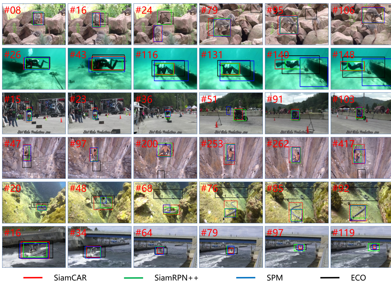
Fig. 5 Examples of tracking results. We show some visual tracking results of three popular trackers SiamRPN++ (Li et al., 2019), SPM (Wang et al., 2019), ECO (Danelljan et al., 2017) and the proposed algorithm on six challenging sequences from GOT-10K (from top to bottom: GOT-10K_Test_60 , GOT-10K_Test_86 , GOT-10K_Test_91 ,
