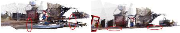
Figure 4: 7-objects sequence: without explicit loop closure detection a plain SLAM engine (left) accumulates error over time, whilst the ability to detect Mario allows our technique to also constrain the last and first frames and thus to tear down the global error (right).
