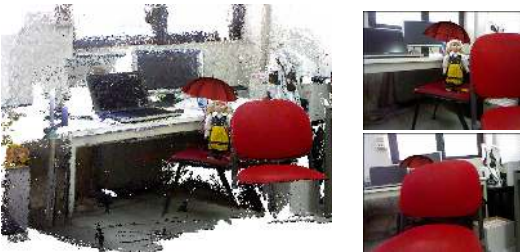
Figure 8: AR with 3D occlusion handling: once the Doll is detected (top right) a red umbrella can be rendered, even when the object is later occluded (bottom right); the final augmented 3D reconstruction is shown on the left.
