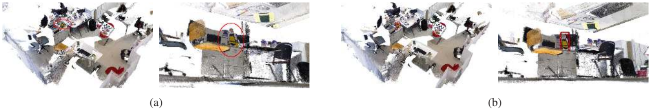
Figure 7: A plain SLAM engine (a) accumulates errors and eventually cannot close the loop; integrated object detection and semantic optimization (b) allows for implicit loop closure and improved reconstruction.
