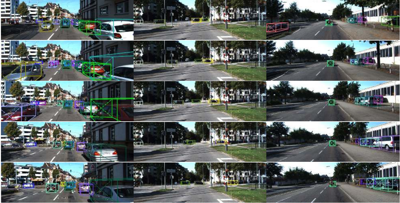
Figure 5: Qualitative results of 3D Estimation on KITTI testing set. We show predicted 3D layout colored with tracking IDs.
