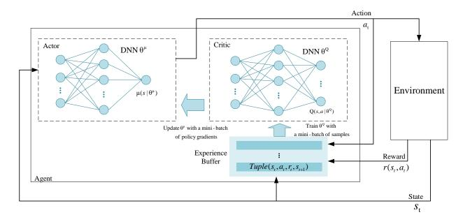
Figure 5. The DDPG algorithm: a model-free, off-policy, and actor-critic algorithm.
