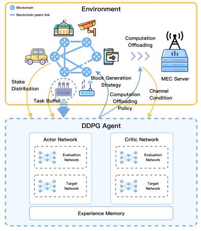
Figure 4. The architecture of the DDPG-based framework.
