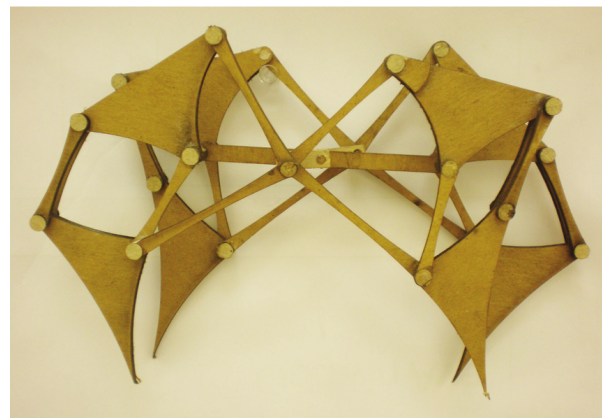
Figure 1. The Jansen's strandbeest can be manufactured by putting together 4 planar linkages to the left and right of the robot's body; see Nansai et al. (2013) for more details.
