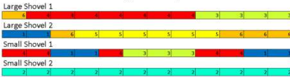
Fig. 6 Comparison of shovel allocation per period (12 months) to mining areas (colour-coded from A1 to A6) for separately optimized production schedule (top) and joint optimization (bottom). (Color figure online)
