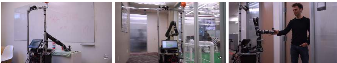
(d) The robot decides which item is a rattling container and grasps it. (e) The robot autonomously navigates to the specified destination room. (f) The robot hands over the item at the specified destination.
