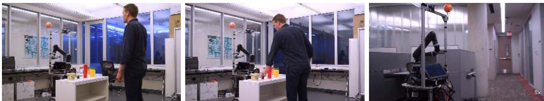
(a) The human says to move a rattling container from one room to another. (b) The robot asks questions about local items to learn the new rattling property. (c) The robot autonomously navigates to the specified location to search for the object.
