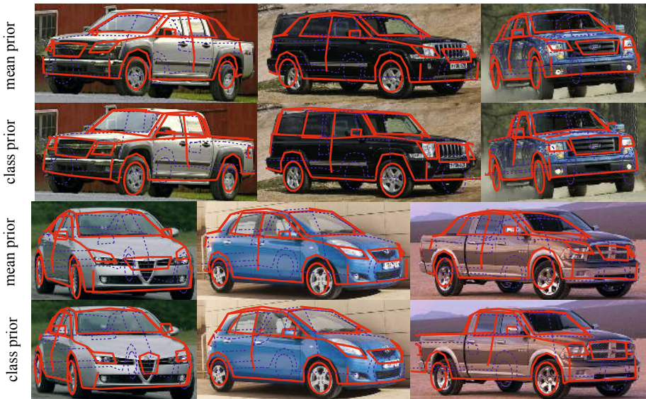
Fig. 7. Comparison of model fitting results. Top row shows the output of mean prior+pose+shape, and the bottom shows our final fitting results: class prior+pose. Our approach can produce better fitting results (e.g., the backside of pickup truck, SUV, hatchback and the grille part of Alfa romeo) compared to the mean prior, because it can more closely match to the target shape (benefiting from the predicted class label) and avoids falling into local minima for our non-linear objective function.
