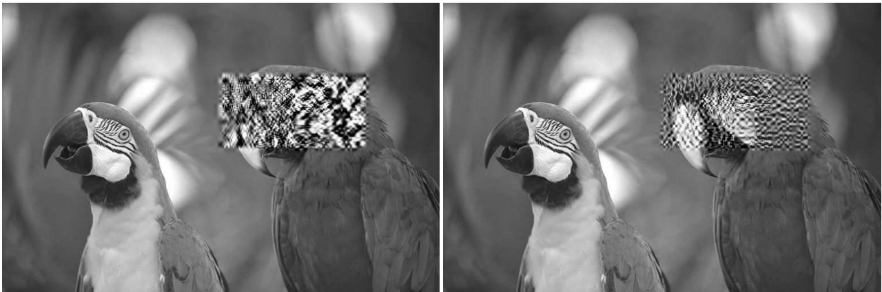
Figure 13 – Scrambling results (left: all layers and resolutions have been scrambled, right: layers 2 and 3 and resolution levels 1 to 3 have been scrambled).
