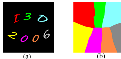
Figure 12: Applying JFA on (a) the input image, we have (b) the result of the generalized Voronoi diagram of the seven area seeds.
