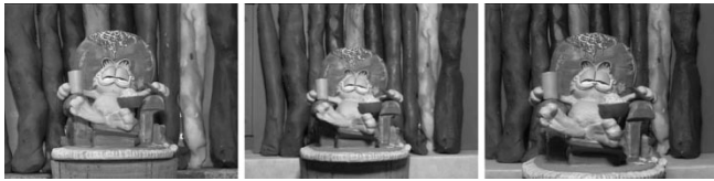
Fig. 1. “Garfield” photographed with telephoto, normal, and wide-angle lenses, from corresponding (a) far, (b) intermediate, and (c) near distances. [View in color at http://www.cs.cmu.edu/~mws/ieee3dvt99 .]
