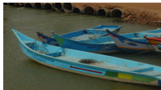
Figure 7. Jute composite boat with outer coating
