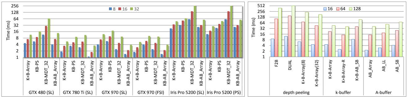
Fig. 9: Performance evaluation in ms ( \log_2 scale) of (left) k -buffer alternatives on different graphics hardware and syncing implementations and (right) depth peeling and A-buffer alternatives on scenes with varying n .
