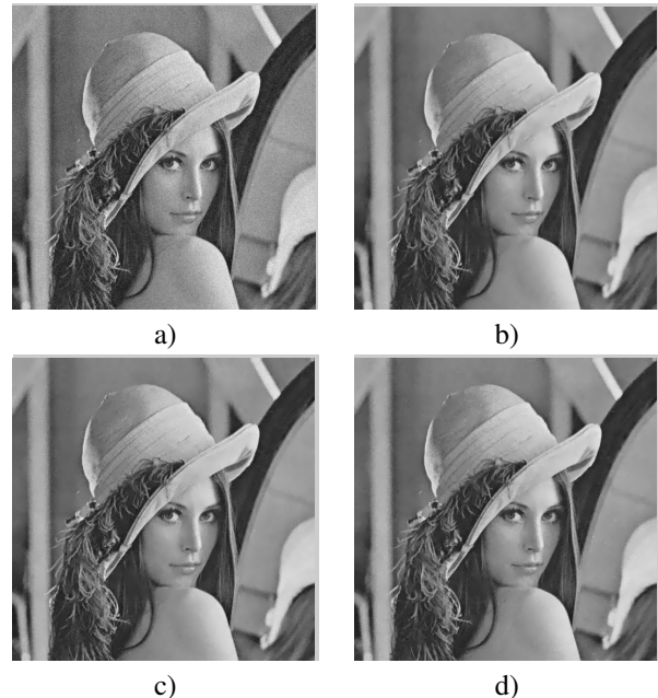
Fig. 2: Denoised images for \sigma = 10 : a) Noisy image (PSNR = 28.12dB), b) Transform K-SVD (PSNR = 33.61dB), c) Analysis K-SVD (PSNR = 33.34dB), d) FD (PSNR = 33.01dB).
