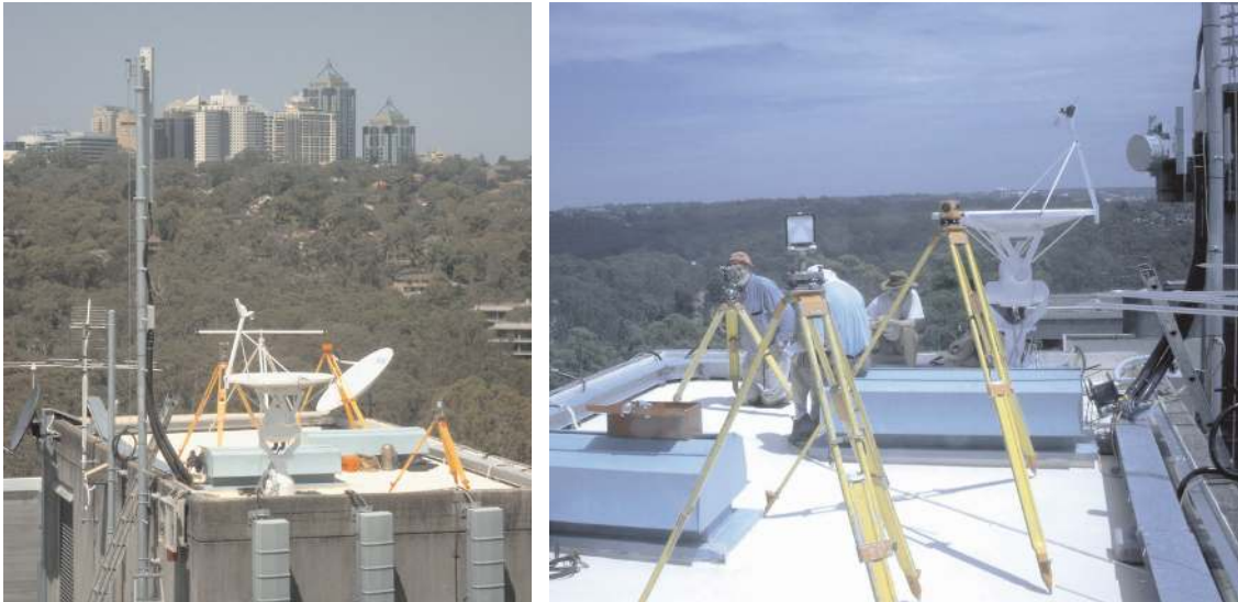
Figure 4.32: Photos of the precision surveying campaign: overview of the location (left) and equipment (right). Some of the obstructing towers and masts can also be seen here.
