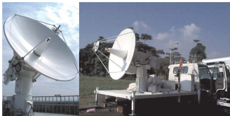
Figure 2.13: Photos of the remote and the transportable terminals for ROCSAT [47]
