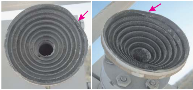
Figure 7.7: Feed horn deformation after a mechanical failure of one of the supporting structures due to gale-force winds
