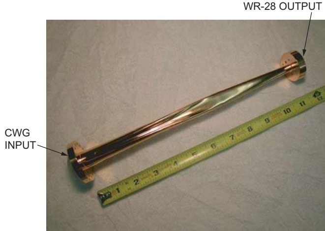
Fig. 6. Prototype of the Marie-mode transducer.
