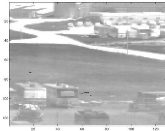
Fig. 15. Corrected version of the image in Fig. 10 using the gain and the bias corresponding to data set 1. Note that less NUC is achieved in comparison with that in Fig. 11 because of the drift in the gain and the bias. Also note that there is no compensation for the dark spots (dead pixels) that appear in Fig. 10.
