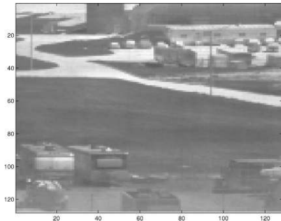
Fig. 8. NUC with 1000 consecutive frames. Note the improvement in comparison with Fig. 7.
