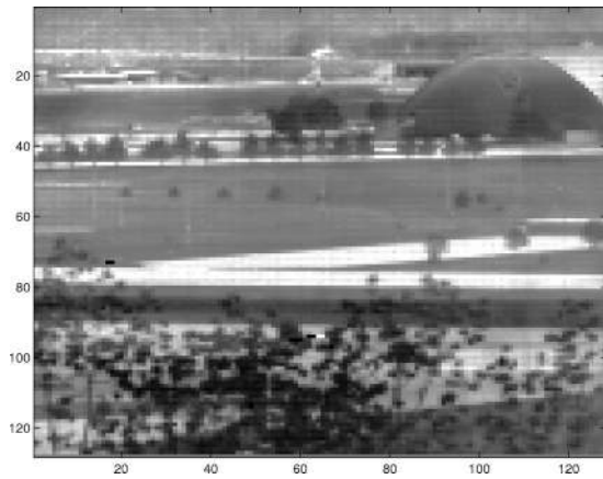
Fig. 14. Corrected version of the image in Fig. 12 using 300 consecutive frames. The drift parameters are assumed as \alpha = \beta = 0.05 , which corresponds to strong drift.
