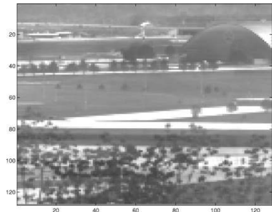
Fig. 13. Corrected version of the image in Fig. 12 using 300 consecutive frames. The drift parameters are assumed as \alpha = \beta = 0.95 , which corresponds to weak drift.
