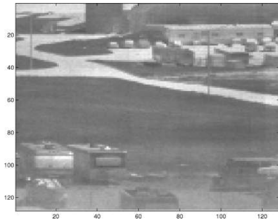
Fig. 7. NUC with 150 consecutive frames. Note the improvement in comparison with Fig. 6; however, some residual artifacts remain, again as a result of a minor violation of the constant-range assumption.
