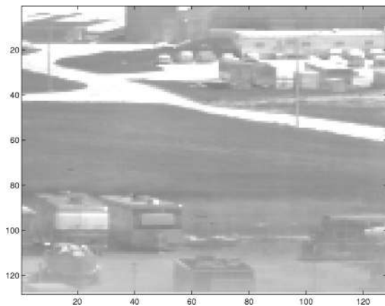
Fig. 11. Corrected version of the image in Fig. 10 using 300 sampled frames. The drift parameters are assumed as \alpha = \beta = 0.95 .
