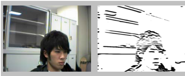
Fig. 5. A typical image and its Gabor filtered image ( \alpha=\pi/2 )
