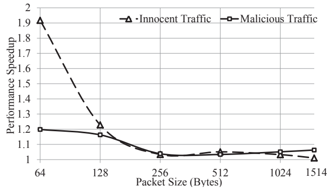
Figure 5: Speedups with function call batching. The input rate is 40 Gbps with innocent and malicious traffic
