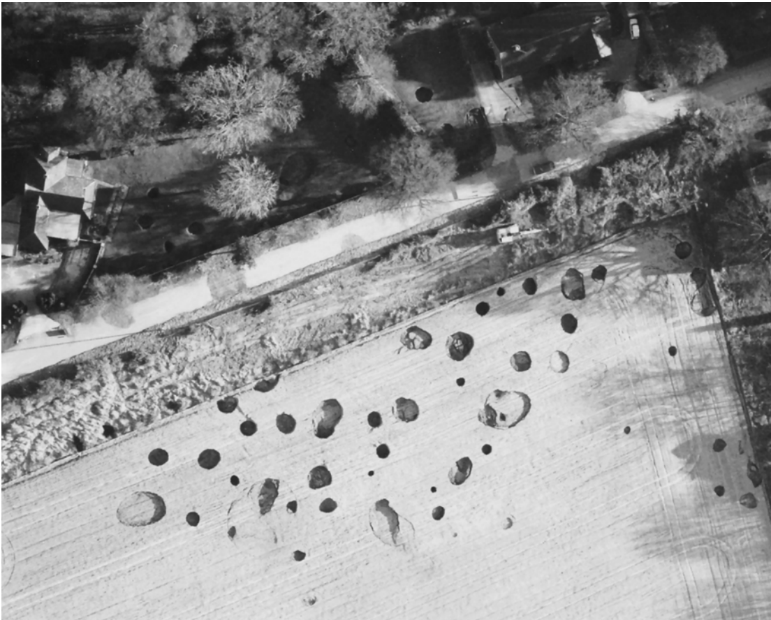
Fig. 8. Numerous sinkholes formed by a large burst water main at Littleheath Road, Fontwell, Sussex [SU 944 077] in late 1985. At least 63 collapses are visible, 8 in gardens, 4 on the road and the remainder in the field. The burst water main was near the digger in the top right of the view. The site is on solifluction deposits overlying Culver Chalk, close to the Palaeogene margin. Photo copyright Sealand Aerial, Chichester, reproduced under licence.
