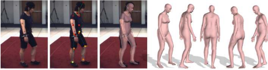
Fig. 2. System overview. Left to right: Given a single image, we use a CNN-based method to predict 2D joint locations (hot colors denote high confidence). We then fit a 3D body model to this, to estimate 3D body shape and pose. Here we show a fit on HumanEva [41], projected into the image and shown from different viewpoints. (Color figure online)
