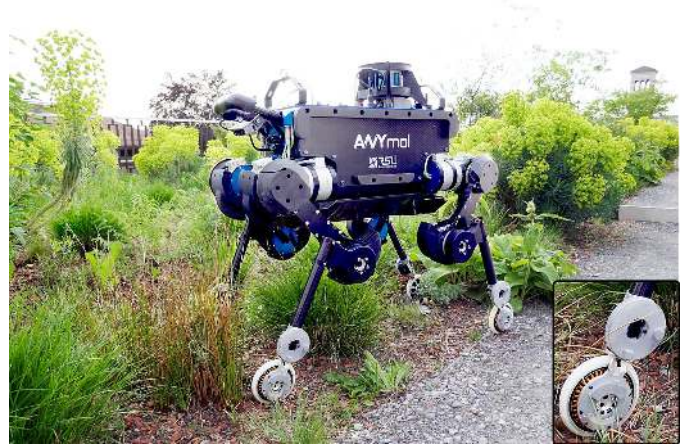
Fig. 1. The fully torque-controlled quadrupedal robot ANYmal [2] is equipped with four non-steerable, torque-controlled wheels. Thus, the number of actuated joint coordinates n_\tau and the number of joints n_j are both equal to 16. A video demonstrating the results can be found at https://youtu.be/nGLUsyx9Vvc .
