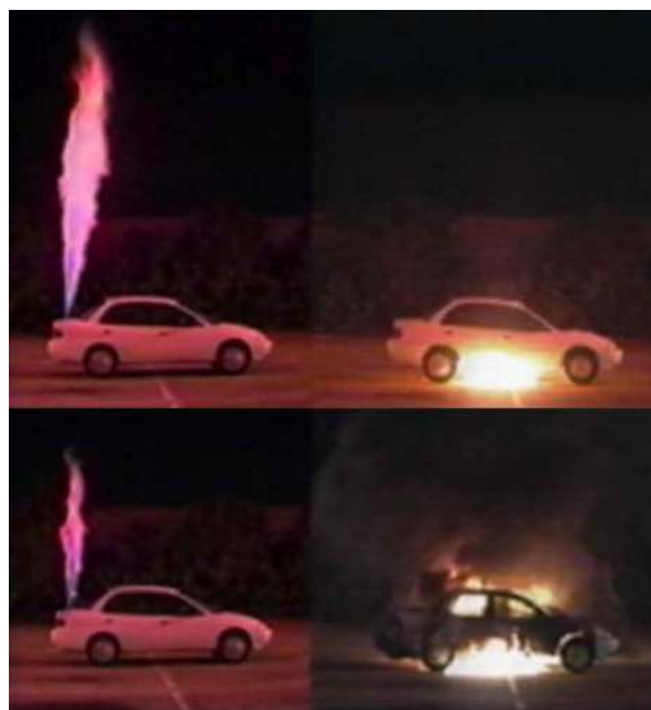
Fig. 6. On the left is a vehicle with a hydrogen tank, and on the right a vehicle with a standard gasoline tank. Both tanks have been deliberately punctured and ignited. The top panel shows the two vehicles 3 seconds after ignition. We see that, due to the buoyancy of hydrogen, the flame shoots up vertically, whereas gasoline is heavy and spreads beneath the vehicle. The bottom panel shows the two vehicles 60 seconds after ignition. The hydrogen supply has burned off and the flame is diminished, whereas the gasoline fire has accelerated and has totally engulfed the vehicle on the right. Note that hydrogen flames are not intrinsically visible, but salt and particles in the ambient air burn off giving color to the flame as seen above. Source: University of Miami.
