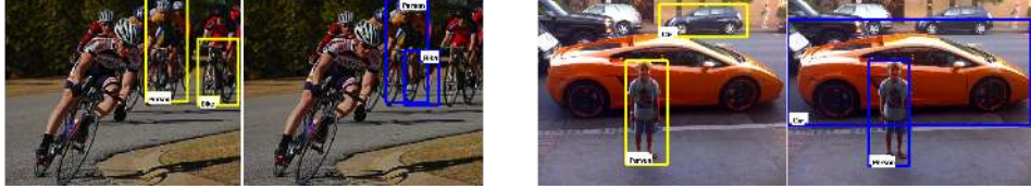
Figure 3: Visualization of how latent variables (i.e. object locations) change during the learning. The left image is from the “person riding a bicycle” category, and the right image is from the “person next to a car” category. Yellow bounding boxes corresponds to the initial object locations. The blue bounding boxes correspond to the object locations after the learning.
