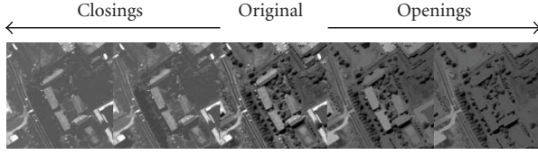
FIGURE 1: Simple morphological profile with 2 openings and 2 closings. In the profile shown, circular structuring elements are used with radius increment 4 ( r = 4, 8 pixels). The image processed is part of Figure 4(a).
