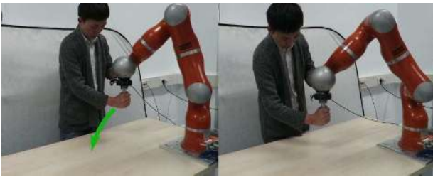
Figure 6. Kinesthetic teaching of the reaching task on the KUKA robot, where demonstrations comprising time and end-effector Cartesian position are collected. The green arrow shows the motion direction of the robot.
