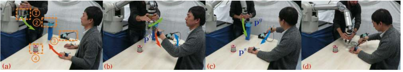
Figure 10. The collaborative hand task in the soldering environment with the Barrett WAM robot. (a) shows the initial states of the user hands and the robot end-effector (the collaborative hand in this experiment). ①–④ separately correspond to the circuit board (held by the robot), magnifying glass, soldering iron and solder. (b) corresponds to the handover of the circuit board. (c) shows the robot grasping of the magnifying glass. (d) depicts the final scenario of the soldering task using both of the user hands and the robot end-effector. Red, blue and green arrows depict the movement directions of the user left hand, right hand and the robot end-effector, respectively.
