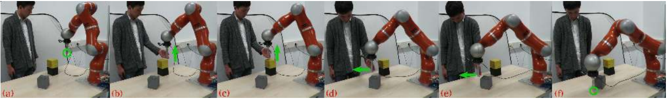
Figure 8. Snapshots of the force-based trajectory adaptations, where the force exerted by the human is used to determine the via-points for the robot, which ensures collision avoidance. (a) and (f) correspond to the initial and final states of the robot, where circles depict the initial and final positions, respectively. Figures (b)–(e) show human interactions with the green arrows depicting the directions of corrective force.
