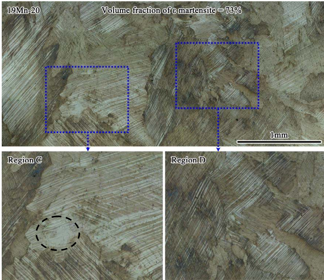
Fig. 6 Color optical micrographs of as-cast 19Mn-20 alloy annealed at 873 K for 30 min after 10% tensile deformation at M_s + 10 K.
