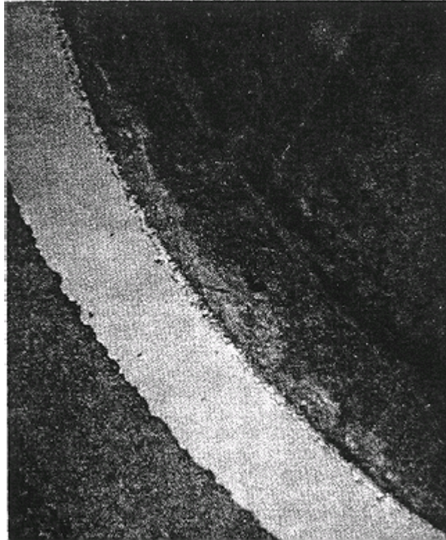
Figure 3-13. Photomicrograph of a UCO particle (batch 6157-08-020) from Compact 10 irradiated at 1040°C to 27.8%FIMA and to a fast fluence ( E>0.18 MeV) of 7.1 \times 10^{25} n/m 2 displaying fission product attack of the SiC layer.
