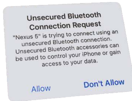
Fig. 8. iPhone notification to mitigate our downgrade attacks. If the user presses Allow, then all the subsequent secure connections with the Nexus 5 can use session keys with entropy values between 1 and 16 bytes. The image is adapted from https://twitter.com/seemoolab/status/1169363042548760577/photo/1 .
