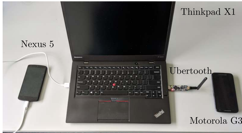
Fig. 4. Our attack scenario for Bluetooth (legacy security) and BLE. In the Bluetooth case, we use a Nexus 5 both as a victim and as the attacker, a Motorola G3 as a victim, and a Thinkpad X1 laptop to patch the Nexus 5’s Bluetooth firmware. In the BLE case, we use a Thinkpad X1 both as the attacker and as a victim. The laptop runs our custom Linux kernel and user-space BLE stack. We eavesdrop Bluetooth and BLE packets using an Ubertooth One.
