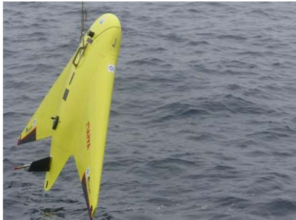
Fig. 13 The ROBEX Glider – a blended wing design for extended operating ranges and long-term deployments (from Waldmann et al. (2016))
