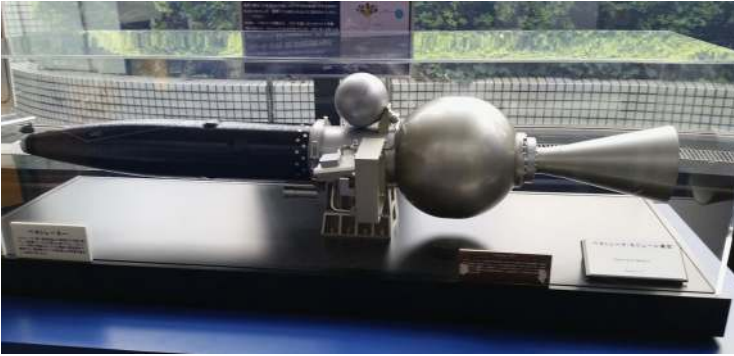
Fig. 5 Model of one of the Lunar-A penetrators, never flown. Only the black element at left would penetrate into the regolith to perform seismic and heatflow studies: the formidable propulsion and attitude control hardware necessary to orient and decelerate the vehicle to survivable impact speed is evident at right, Photo: R. Lorenz
