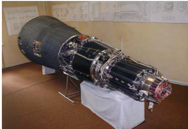
Fig. 15 Nuclear power plant with thermionic reactors for space applications “Topaz” (from Kraus and Shabalín (2013))
