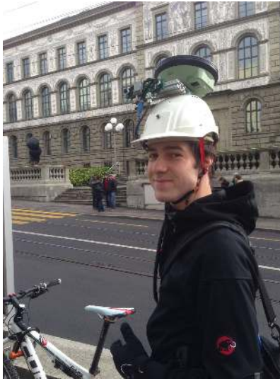
Fig. 14. Simon Lynen ready for dataset collection on a bicycle at ETH with sensor and GNSS ground-truth recorder mounted to a helmet.
