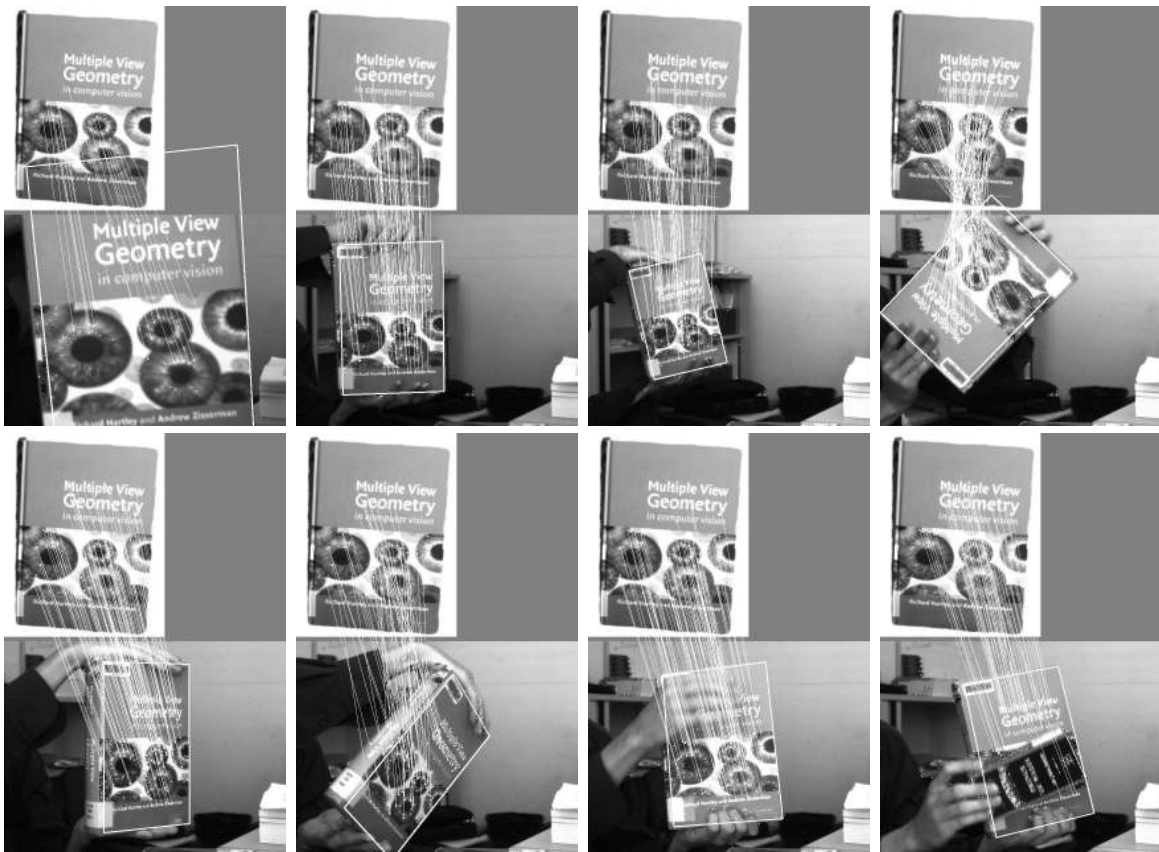
Fig. 15. Detection of the book: The white lines represent the inlier matches established in real-time under several poses. The corresponding video sequence is submitted as supplementary material.
