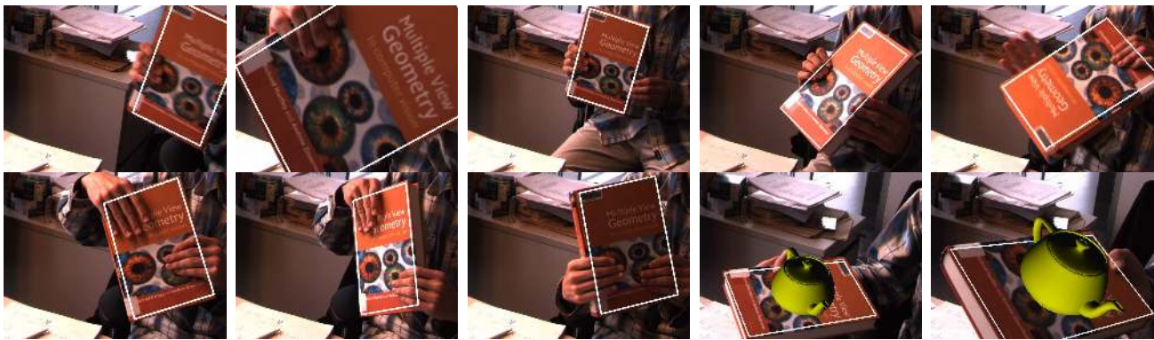
Fig. 1. Detection of a book in a video sequence: As shown by the white outline, the book is detected independently and successfully in all frames at 25Hz in 640 \times 480 images on a standard PC, in spite of partial occlusion, cluttered background, motion blur, large illumination and pose changes. In the last two frames, we add the inevitable virtual teapot to show we also recover 3-D pose. The corresponding video sequence is submitted as supplementary material.
