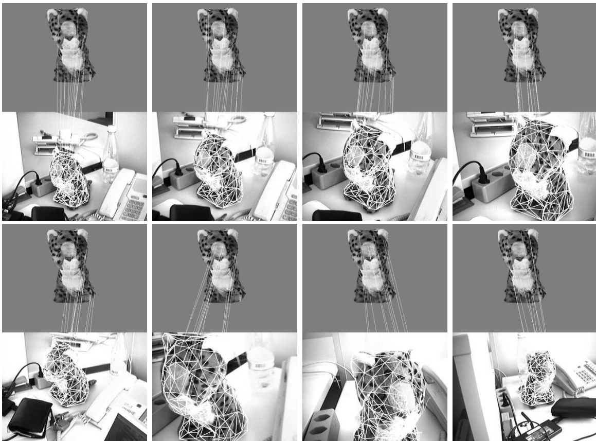
Fig. 18. Our method can take advantage of a 3-D model when available, to detect the target and estimate its pose from different viewpoints.
