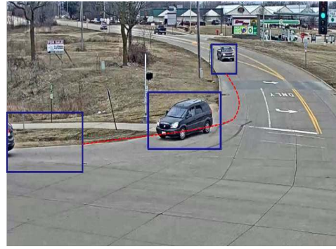
Figure 3. An example of matching a query to video frames of a vehicle. For specifying a vehicle, we use four criteria. The order of the video frames is left to right.
