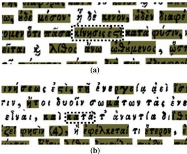
Fig. 11 Examples of wrongly segmented words: a word image merging; b single word image splitting
