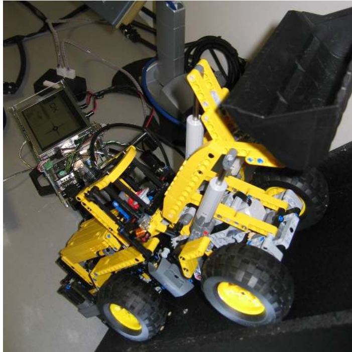
Figure 13. A Lego model of a wheel loader used for test case execution in the MOGENTES project.
