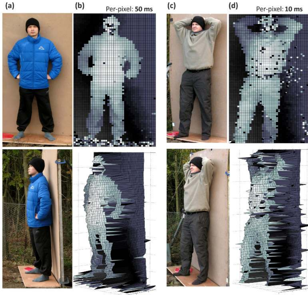
Fig. 6. Depth profile measurements of humans, acquired in daylight at a standoff distance of 910 meters. The close-up photographs in columns (a) and (c) are different viewpoints of the scenes which were scanned – two of the authors posed in front of a sheet of hardboard. The depth scans were acquired in bright daylight and each scan covered an area of approximately 800 \times 2000 mm using 40 \times 80 pixels, corresponding to a maximum field of view of 2 mrad. Surface plots of the raw depth data obtained are shown in columns (b) and (d) - these columns show two different views of the data obtained with the specified per-pixel dwell time. It took 32 seconds to acquire the data shown in (d). The color shading in the surface plots is used to map depth.
