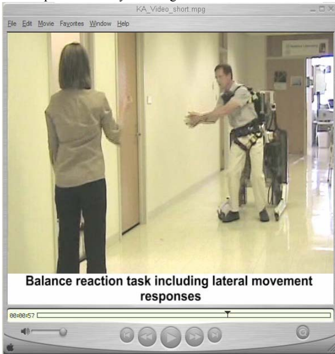
Fig. 4. A still image from a 35 second silent movie showing the KineAssist in action. The movie may be found at www.chicagopt.com/info The movie shows (1) patient rising from sit to stand, assisted or freely allowed by the KineAssist. (2) patient walking, showing free hip and torso motions about several axes (3) physical therapist assisting with patient's legs during gait. Note that the clinician's chair is pulled along by the KineAssist. (4) patient's side stepping and torso motions to allow reaching and balance (5) patient tripping and falling and being caught by the KineAssist. (The patient in the movie is a healthy individual. Both the patient and the physical therapist are employees of Chicago PT LLC.)
