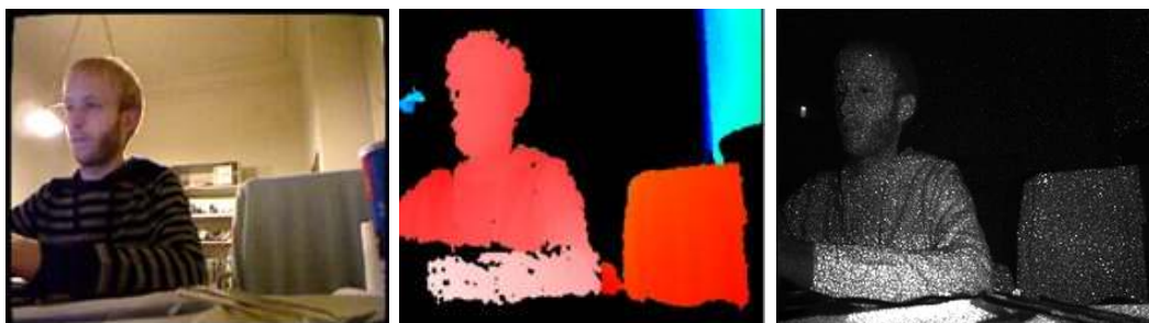
Figure 4.2: Kinect provided data: RGB image (left), depth (middle) and infrared image (right).
