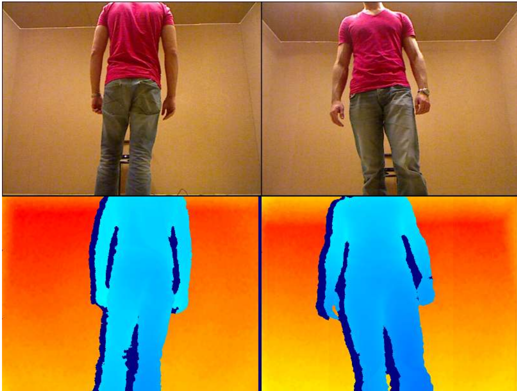
Figure 4.18: The figure shows the RGB images (top) and depth images (bottom) from two Kinects recorded simultaneously. The setup is as shown on figure 4.17.
