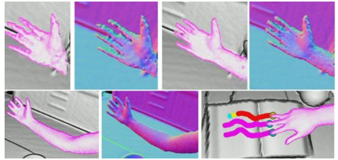
Figure 16: Segmentation, tracking and reconstruction of user's arm with moving Kinect. Top left: Arm is first introduced and reconstruction contains a great deal of noise. Top right: surface is refined based on separate ICP-based pose prediction. Bottom left: the moving surface is rapidly reconstructed to a much higher quality than the raw Kinect signal. Bottom right: The intersection between foreground and background surfaces are used for multi-touch detection.
