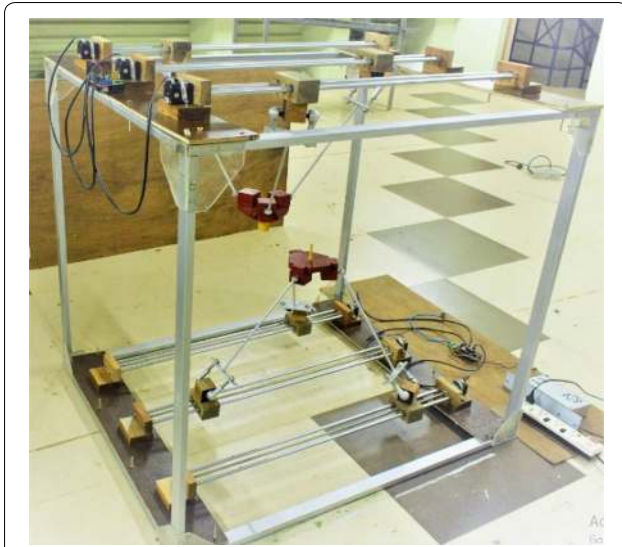
Figure 18 Experimental setup of 3-PRUS dual PKM prototype
