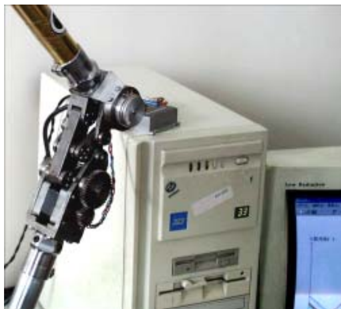
Figure 14. Six-bar mechanism knee for experiment.
