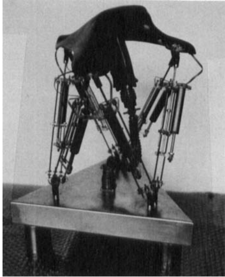
Figure 7. Second prototype. The mechanism has been rotated by 90^\circ , resulting in a horizontal mobile platform (see text). The problem of connecting the handle to the six legs has been solved by a molded piece that is made light and rigid. At the same time, a clean line provide an unambiguous sense of orientation at a glance, increasing the comfort of utilization.
