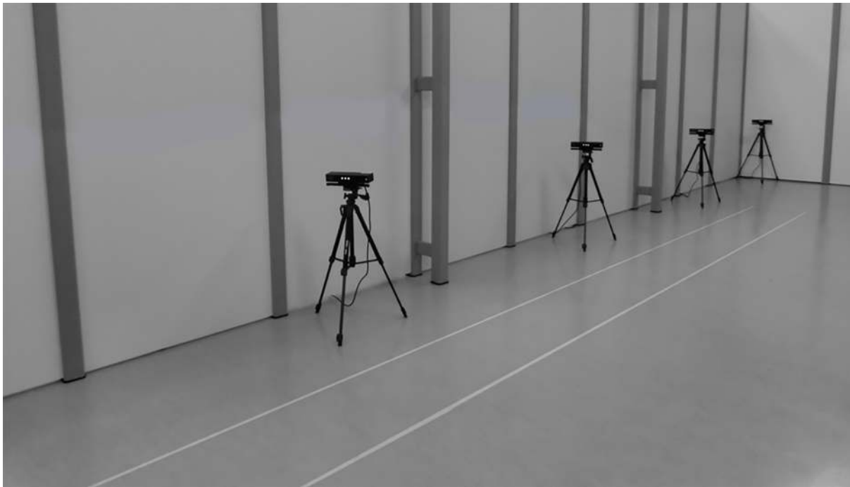
Fig 2. Overview of the multi-Kinect v2 set-up.
