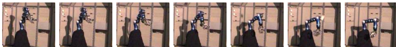
Fig. 10. Image sequence (from upper left to lower right) for “latest” mode catching with \Delta t = 120ms (same throw as in Fig. 9) and t \approx 0s for the first and t \approx t_{c,latest} + 20ms = 0.72s for the last image.
