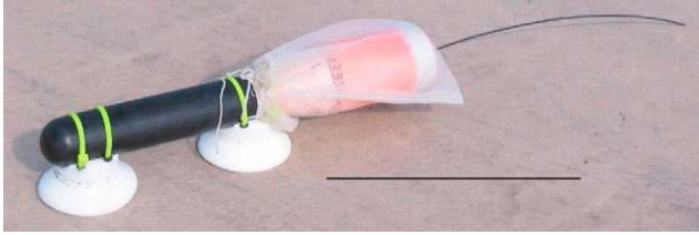
Fig. 1. Bioacoustic probe. The high-resolution digital tag contains a depth gauge, a two-axis accelerometer and a hydrophone (Bioacoustic Probe; Burgess et al., 1998). The tag was harnessed with silicon suction cups for attachment and a flotation device for retrieval. Scale bar, 20 cm.
