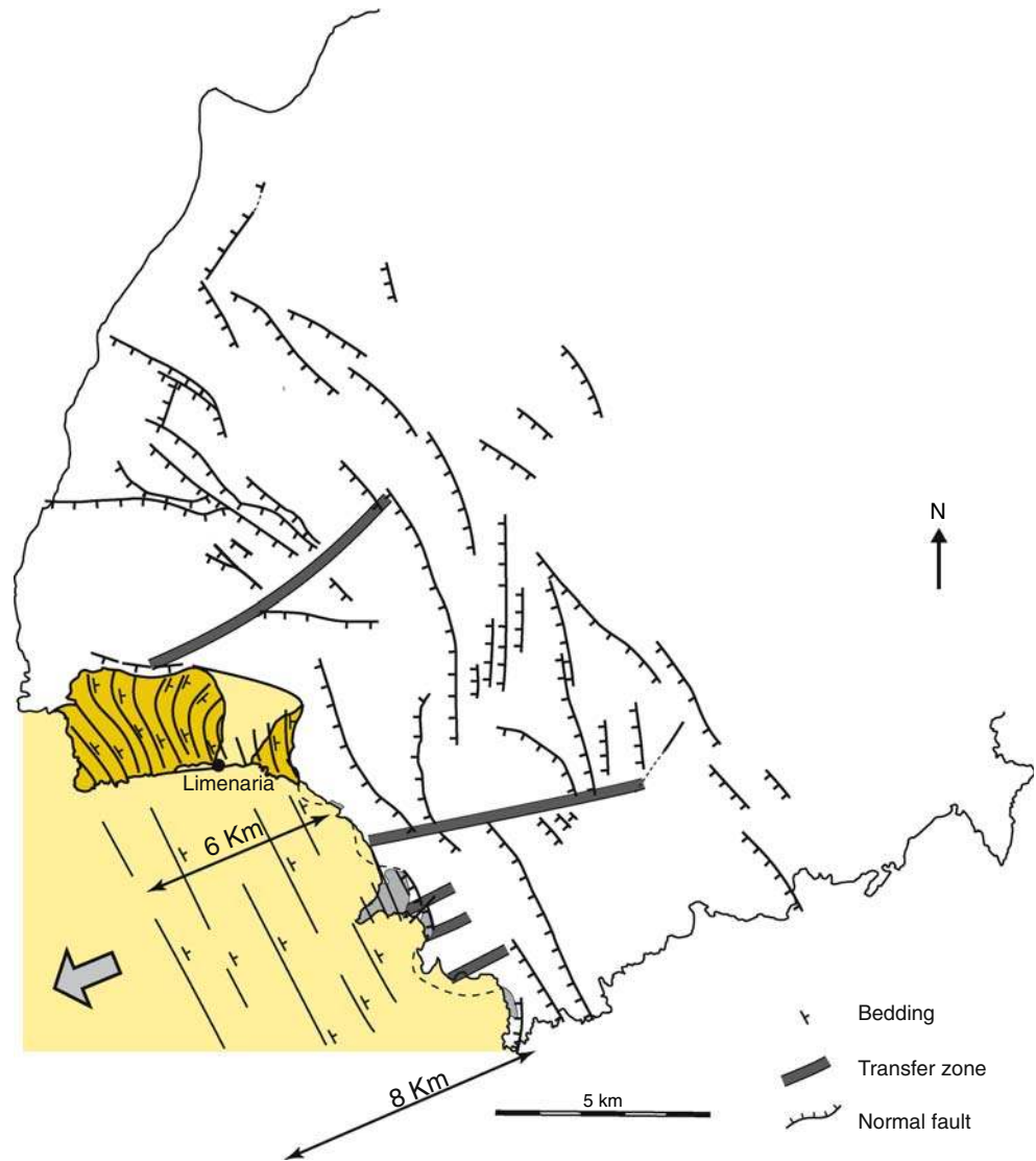
Fig. 11 Map of the Limenaria Basin with bedding trends, normal faults and transfer zones
