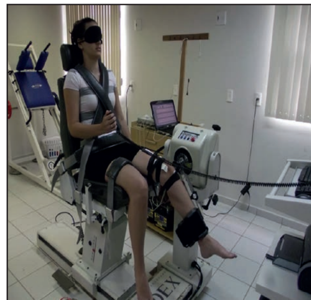
Figure 02. Positioning of the volunteer on the isokinetic dynamometer (Biodex Multi-Joint System 3®, Biodex System Biomedical Inc, New York, USA) for evaluation of the JPS.
